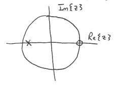
Passband is centered at w= TT due to pole at ==-0.9. Stopband is centered at w=0 due to zero at Z=1. Highpass filter.
