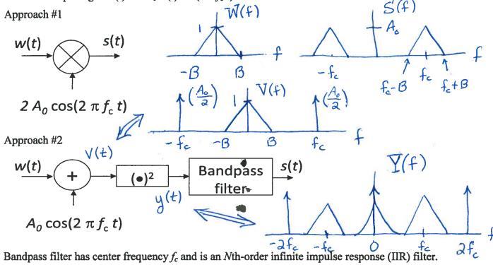
Bandpass filter has center frequency  $f_c$  and is an Nth-order infinite impulse response (IIR): Baseband message signal w(t) has bandwidth B where  $f_c > 2$  B.  $f_c > 3$  B.
