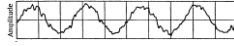
C Modulation carries the encoded sine wave information, as can be seen after 32 averagings.
