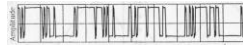
B Dither of one-third LSB rms amplitude is added to the sine wave before quantization, resulting in a PWM waveform.
