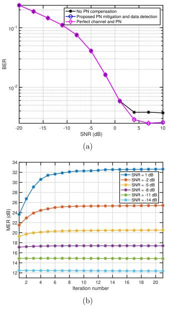
Figure 4.17: Evolution of the BER versus SNR (a) and MER versus number of iterations in the proposed PN mitigation and data detection algorithm (b), for SNR =  $\{-14, -11, -8, -5, -2, 1\}$  dB before beamforming, using a 256-QAM constellation and  $N_{\rm s}=2$  data streams.
