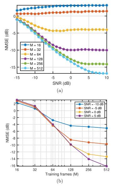
Figure 3.8: Evolution of the NMSE achieved by the joint synchronization and channel estimation algorithm as a function of SNR (a) and M (b). The number of training frames is  $M = \{16, 32, 64, 128, 256, 512\}$ , and the length of the time-domain training sequence is N = 128.
