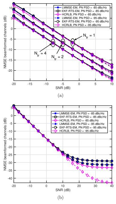
Figure 4.8: Evolution of the NMSE of the beamformed channel estimates obtained using the proposed algorithms versus SNR. The hybrid CRLB is also provided as a performance bound.
