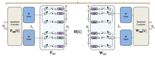
Figure 4.2: Illustration of the structure of a partially-connected hybrid MIMO architecture, which includes analog and digital precoders and combiners (same as Fig. 1.3).
