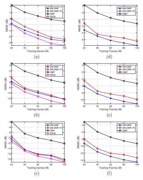
Figure 2.8: Comparison of evolution of the NMSE versus M at different SNR. The SNR is set to -10 dB (a) and (d), -5 dB (b) and (e) and 0 dB (c) and (f). Plots (a), (b), (c) consider on-grid angular parameters on the channel realizations, while (d), (e), (f) consider the off-grid case with channel realizations extracted from the NYUSIM channel simulator [4].
