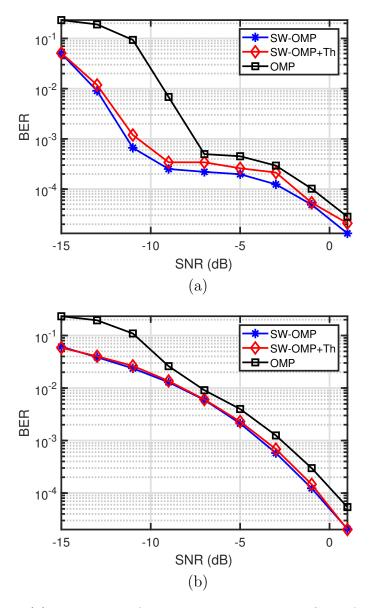
Figure 2.10: (a) Evolution of the coded BER versus SNR for the different frequency-domain algorithms. The number of training frames is set to M=60. (b) Evolution of the uncoded BER versus SNR for the different frequency-domain algorithms. The number of training frames is set to M=60.
