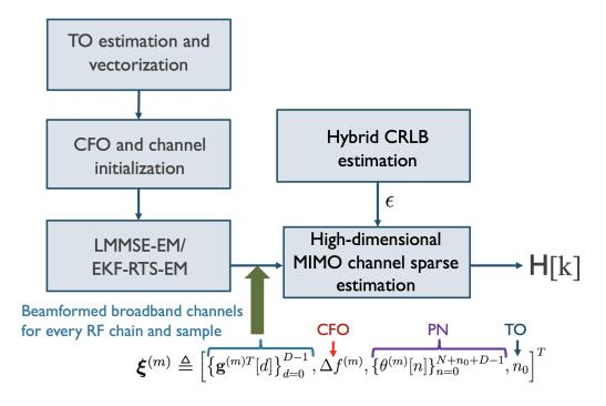
Figure 4.3: Block diagram of the proposed estimation-theoretic framework for joint synchronization and compressive channel estimation under broadband mmWave MIMO channels.
