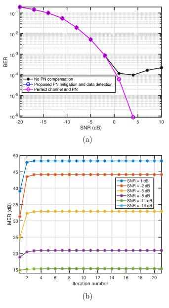
Figure 4.16: Evolution of the BER versus SNR (a) and MER versus number of iterations in the proposed PN mitigation and data detection algorithm (b), for SNR =  $\{-14, -11, -8, -5, -2, 1\}$  dB before beamforming, using a 64-QAM constellation and  $N_{\rm s}=2$  data streams.
