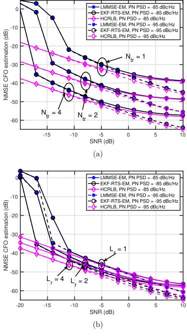
Figure 4.6: Evolution of the NMSE of the CFO estimates obtained using the proposed algorithms versus SNR. The hybrid CRLB is also provided as a performance bound.
