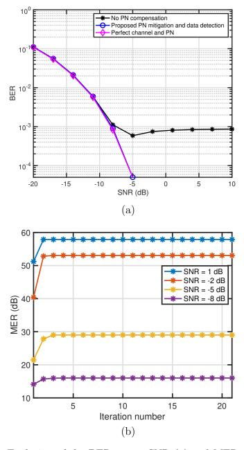
Figure 4.15: Evolution of the BER versus SNR (a) and MER versus number of iterations in the proposed PN mitigation and data detection algorithm (b), for SNR =  $\{-14, -11, -8, -5, -2\}$  dB before beamforming, using a 16-QAM constellation and  $N_{\rm s}=2$  data streams.
