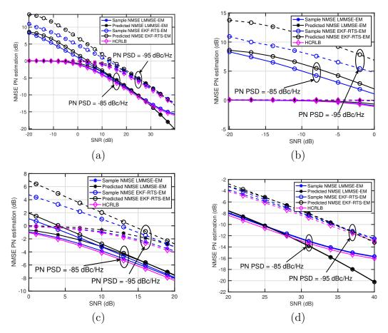
Figure 4.10: Asymptotic evolution of the NMSE of the PN estimates obtained using the proposed algorithms versus SNR. The curves in (a) show this asymptotic evolution for SNR values between -20 and 40 dB. Magnified curves of the asymptotic evolution are also shown for SNR  $\in [-20, 0]$  dB in (b), SNR  $\in [0, 20]$  dB in (c), and SNR  $\in [20, 40]$  dB in (d). The hybrid CRLB is also provided as a performance bound.
