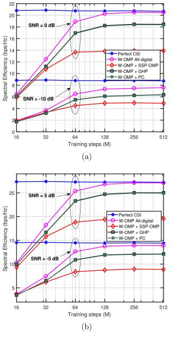
Figure 3.10: Evolution of the spectral efficiency versus M for different precoders and combiners. The number of time-domain training symbols is N=128. The SNR is set to SNR =  $\{-10,0\}$  dB (a) and SNR =  $\{-5,5\}$  dB (b).
