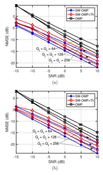
Figure 2.7: Evolution of the NMSE versus SNR for the different frequency-domain algorithms. The number of training frames is set to M=60 (a) and M=100 (b). The channel realizations are taken from NYUSIM channel simulator.
