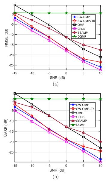
Figure 2.5: Evolution of the NMSE versus SNR for the different frequency-domain algorithms when the AoD/AoA are assumed to lie on the dictionary grid. The number of training frames is set to M=80 (a) and M=120 (b).
