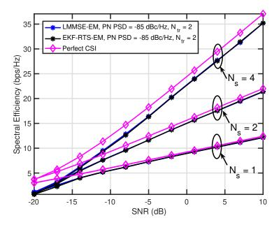
Figure 4.13: Evolution of the ergodic spectral efficiency achieved by the proposed algorithms versus SNR, for  $N_{\rm tr}=2$  OFDM training symbol. The curves are obtained using the 3GPP UMi NLOS channel model [6].
