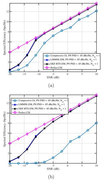
Figure 4.12: Evolution of the ergodic spectral efficiency achieved by the proposed algorithms and the compressive beamforming algorithm in [5] under PN impairments versus SNR, for  $N_{\rm tr}=1$  OFDM training symbol. The curves in (a) are obtained using the mmMAGIC LOS channel model, while those in (b) are obtained using the mmMAGIC NLOS channel model with a Rician factor of  $-10~{\rm dB}$ .
