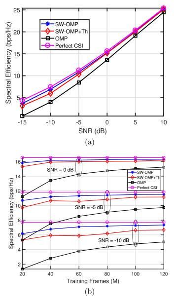
Figure 2.9: (a) Evolution of the spectral efficiency versus SNR for the different frequency-domain algorithms. The number of training frames is set to M=60. (b) Evolution of the spectral efficiency versus number of training frames M at different SNR for the different frequency-domain algorithms.
