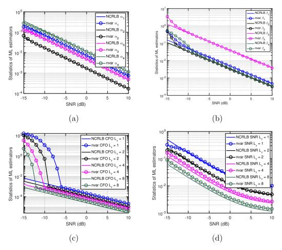
Figure 3.6: Normalized sample variance of the ML estimators from Section 3.4 as a function of SNR. The normalized CRLB is also shown to compare the performance of the ML estimators to the minimum achievable estimation variance. The FFT size of the CFO estimator is set to K = 4N = 1024 points.
