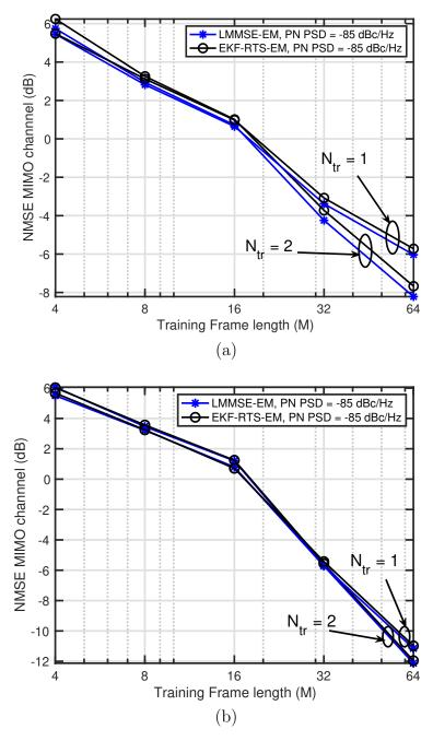
Figure 4.11: Evolution of the NMSE of the mmWave MIMO channel estimates obtained using the proposed algorithms versus M, for SNR = -10 dB (a) and SNR = 0 dB (b).
