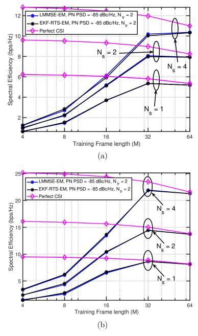
Figure 4.14: Evolution of the ergodic spectral efficiency achieved by the proposed algorithms versus the number of training frames M, for SNR = -10 dB (a) and SNR = 0 dB (b), and  $N_{\rm tr}$  = 2 OFDM training symbols. The curves are obtained using the 3GPP UMi NLOS channel model [6].
