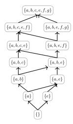
Figure 2 Lattice of Consistent Cuts for Figure 1
