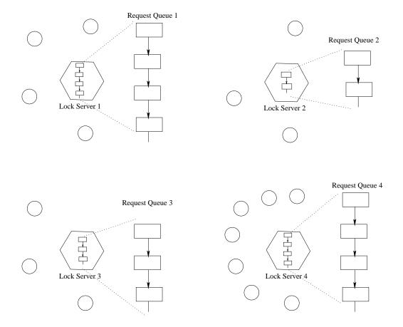
Figure 1.2: System of Four Independent Servers
