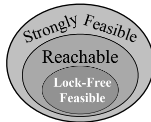
Figure 6.1: The set of lock-free feasible global states and the set of strongly feasible global states are a lower and an upper approximation of reachability, respectively, in a valid loiset.
