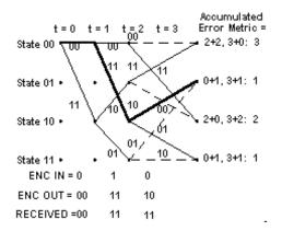
Note that the third channel symbol pair we received had a one-symbol error. The smallest accumulated error metric is a one, and there are two of these.
