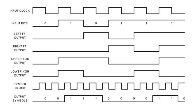
After all of the inputs have been presented to the encoder, the output sequence will be:
