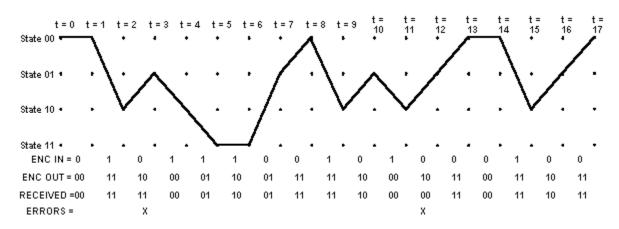
The decoding process begins with building the accumulated error metric for some number of received channel symbol pairs, and the history of what states preceded the states at each time instant t with the smallest accumulated error metric. Once this information is built up, the Viterbi decoder is ready to recreate the sequence of bits that were input to the convolutional encoder when the message was encoded for transmission. This is accomplished by the following steps:
