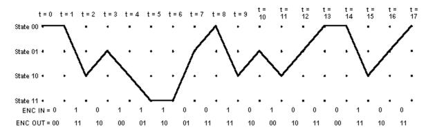
The encoder input bits and output symbols are shown at the bottom of the diagram. Notice the correspondence between the encoder output symbols and the <u>output table</u> discussed above. Let's look at that in more detail, using the expanded version of the transition between one time instant to the next shown below:
