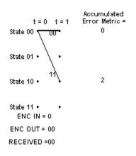
Note that the solid lines between states at t = 1 and the state at t = 0 illustrate the predecessor-successor relationship between the states at t = 1 and the state at t = 0 respectively. This information is shown graphically in the figure, but is stored numerically in the actual implementation. To be more specific, or maybe clear is a better word, at each time instant t, we will store the number of the predecessor state that led to each of the current states at t.
