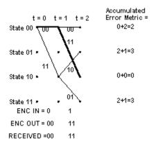
That's all the computation for t = 2. What we carry forward to t = 3 will be the accumulated error metrics for each state, and the predecessor states for each of the four states at t = 2, corresponding to the state relationships shown by the solid lines in the illustration of the trellis.
