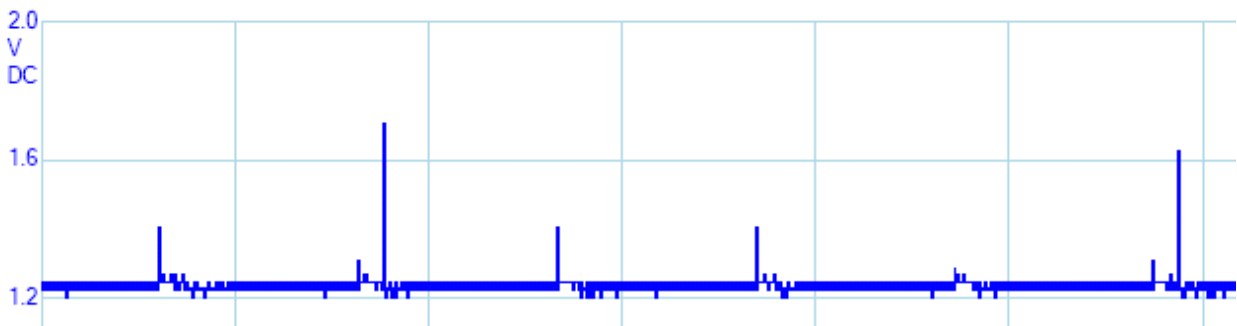
Figure 6.2. GPY0A21YK sensor output, distance=20 cm, DC mode, voltage scale is 0.4 V and time scale is 1 ms.
