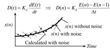
$$D(n) = K_d \left( \frac{1}{2} \frac{E(n) - E(n-3)}{3\Delta t} + \frac{1}{2} \frac{E(n-1) - E(n-2)}{\Delta t} \right) \quad \text{-Analog filter}$$
