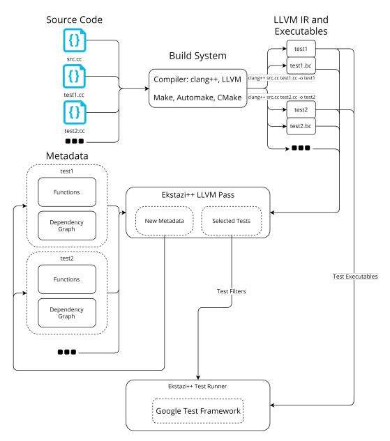
Figure 3.1: Block diagram that illustrates the integration of Ekstazi++ into the workflow.
