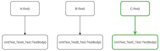
(b) Dependency graph traversal for modified example from C::foo() with the traversal path in green.
