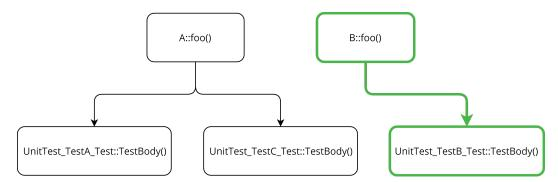
(a) Dependency graph traversal for original example from B::foo() with the traversal path in green.
