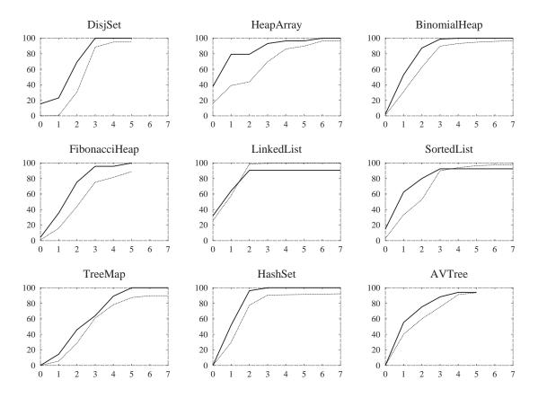
Figure 9: Variation of statement code coverage (thick line) and rate of mutant killing (thin line) with scope. For *all* benchmarks, Korat generates inputs that achieve the maximum coverage that is possible without directly generating inputs for helper methods.
