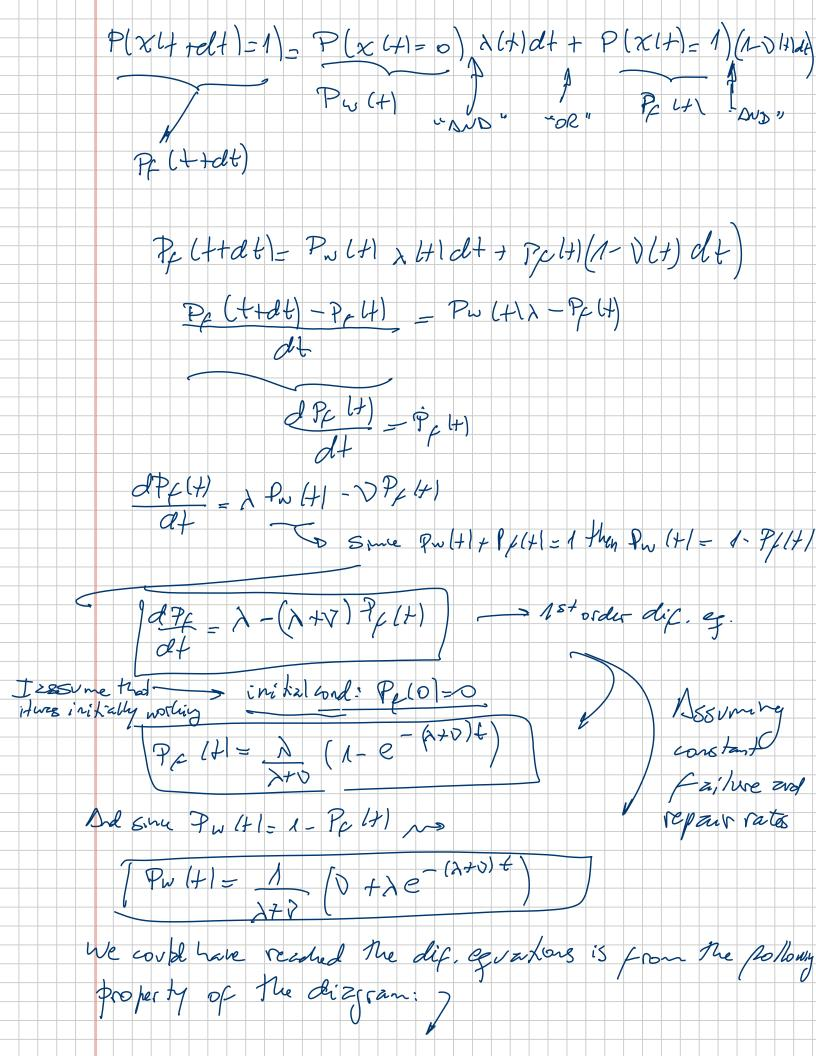
dPstate - (Rate of entering the state) - (Rzto of leaving the state) Interns of Rates, Marhov's diagram becomes: Pw= DP=(+) - X Pw (+) If we plot Pflt ad Pult ) we obtain: Steady state probabilities of sen failed or working. I.e. how likely it is that after having seen there" for a long three the it has it working or not. This fits The definitions of Evailability and Unavailability. Here,
