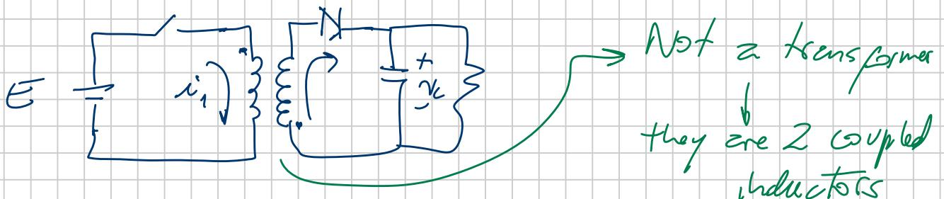
$$\frac{d\phi}{dt} = \frac{V_1}{N_1} = \frac{V_2}{N_2}$$
