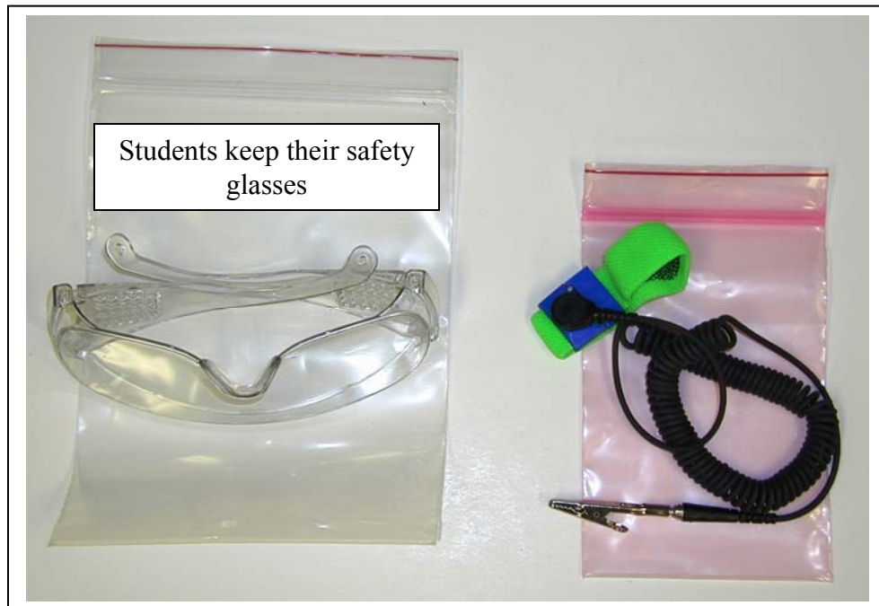
Additional Tools: Safety Glasses and Static Wristband (one per team) Please keep the safety glasses and static wristband in their individual reclosable bags or boxes. The safety glasses' lenses are easily scratched if bagged with tools.
