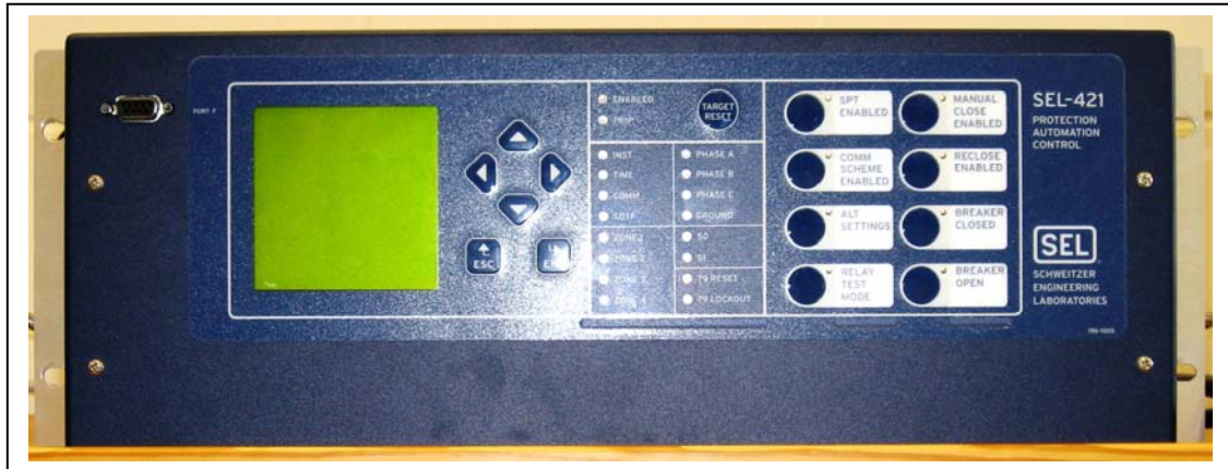
Schweitzer Engineering Labs SEL-421 Relay (the SEL-421 also serves as three-phase meter and event-triggered waveform capture device)
