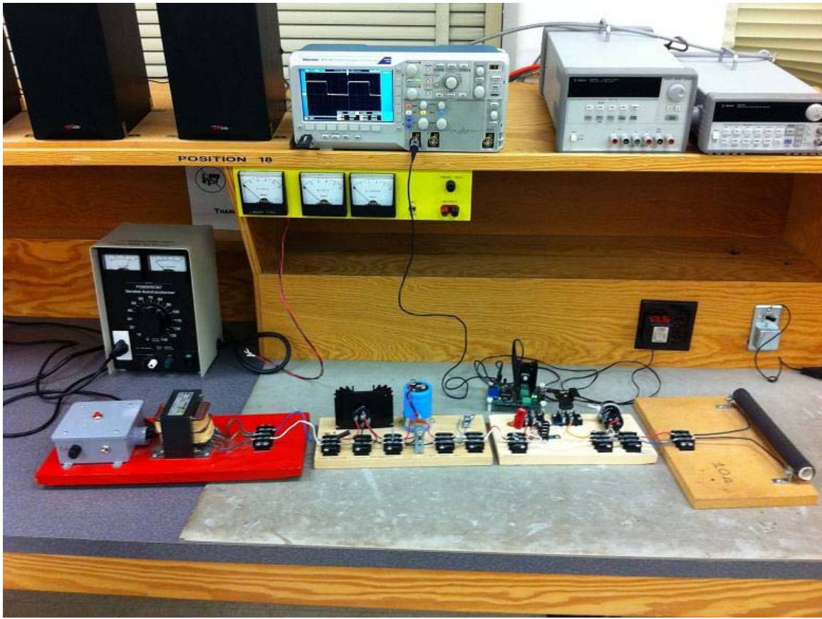
Picture 1: Buck Converter Laboratory Test Setup
