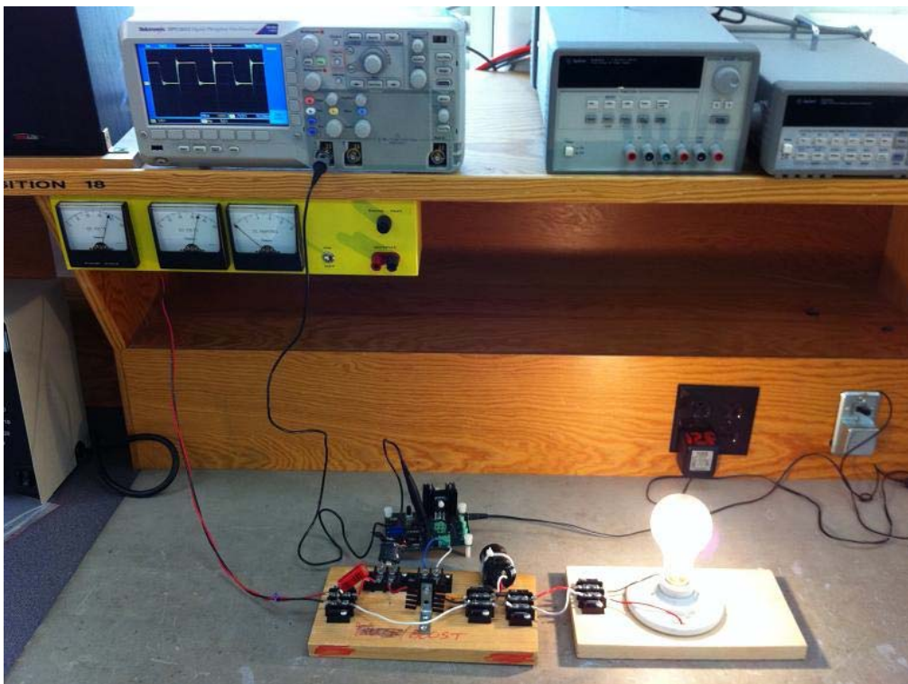
Figure 5: Boost used in conjunction with a solar panel to power a 150 W light bulb load.
