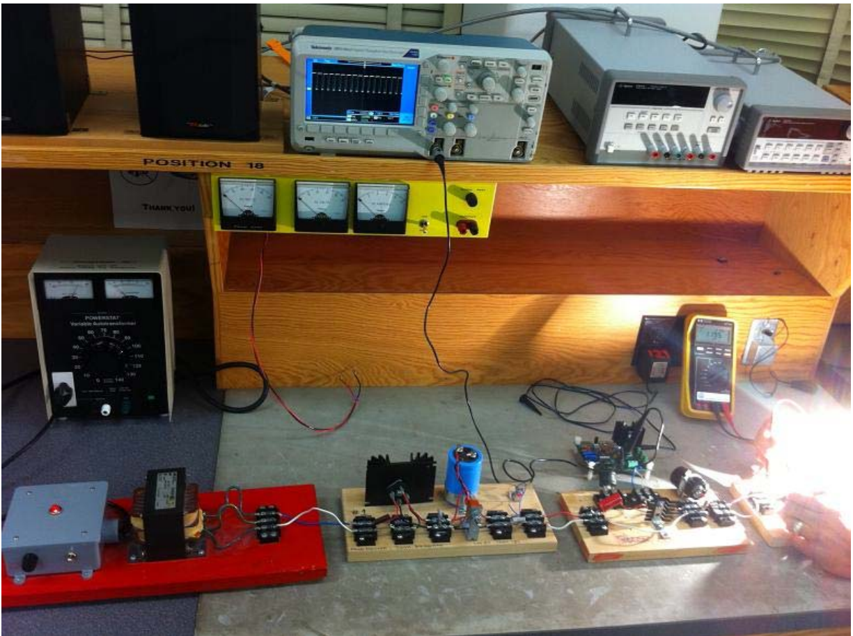
Picture 1: Boost Converter Laboratory Test Setup
