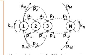
Markov chain model for PV + battery system
