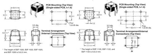
Horizontal, Flat Plunger Type (with Ground Terminal, Pitch: 7.5 mm)
