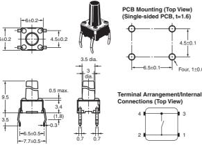
Horizontal, Projected Plunger Type (without Ground Terminal)
