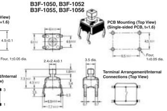
Horizontal, Projected Plunger Type (with Ground Terminal)
