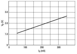
**Figure 6. Clamp Diode Characteristics**
