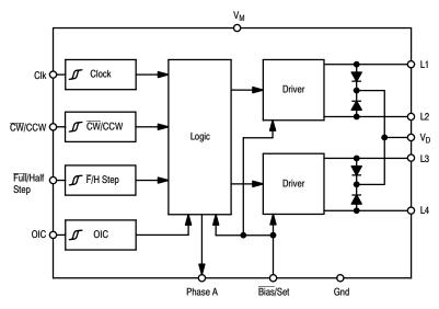
Figure 1. Representative Block Diagram
