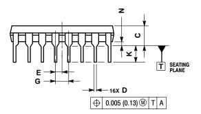
NOTES: 1. DIMENSIONING AND TOLERANCING PER ASME Y14.5M, 1994. 2. CONTROLLING DIMENSION: INCH. 3. DIMENSION I TO CENTER OF LEADS WHEN FORMED PARALLEL 4. DIMENSION B DOES NOT INCLUDE MOLD FLASH.
