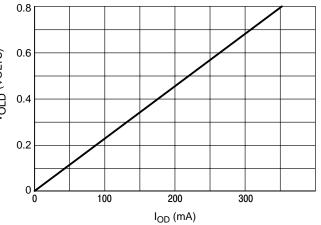
Figure 9. Maximum Saturation Voltage – Driver Output Low
