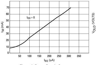
**Figure 8. Power Supply Current**
