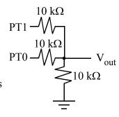
(5) Question 3. What is the output voltage  $V_{out}$  when PT1 is high and PT0 is high? Assume  $V_{OH}$  is 5V and  $V_{OL} = 0V$ .
