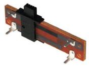
Solder wires to pins 1,2,3 Glue transducer to a solid Position metric ruler (for calibration and testing) Create a hair-line cursor
