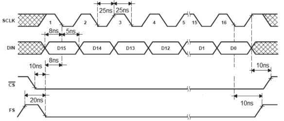
(2) Part a) What is the setup time for the TLV5616? Give the number in ns.
