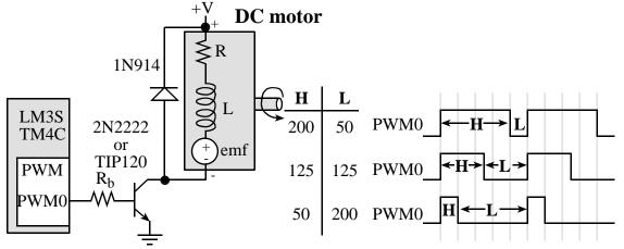
Assume +V is +5V. Let the PWM0 output be high, so the collector voltage of transistor is 0.5V. The transistor is fully in saturation. Is it possible for current to flow up from the collector into the +5V supply? Answer yes or no.
