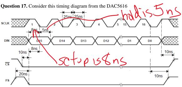
(2) Part a) What is the setup time for the TLV5616? Give the number in ns.
