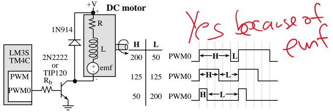
Assume +V is +5V. Let the PWM0 output be high, so the collector voltage of transistor is 0.5V. The transistor is fully in saturation. Is it possible for current to flow up from the collector into the +5V supply? Answer yes pr no.
