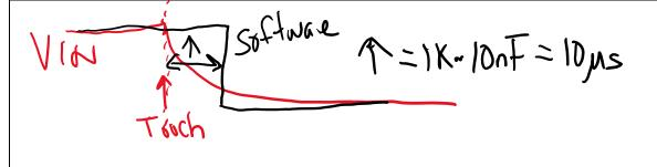
(5) Part c) Assume the switch has been touched for a long time and is released at t=0. Make a rough sketch of  $V_{in}$  versus time. At what approximate time ( $\tau$ ) will the software see the 1 to 0 transition?
