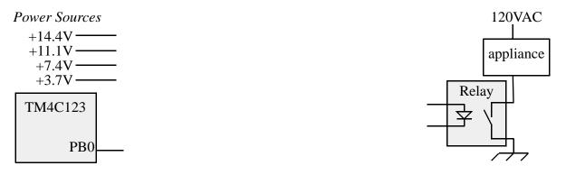
The interface is a simple positive LED interface with no driver. It is ok to pick any  $V_{OH}$  between 2.4 and 3.3 V. At  $V_{OH} = 2.4$ V, R = (2.4-2)/4mA = 0.4V/4mA = 100 ohms. At  $V_{OH} = 3.3$ V, R = (3.3-2)/4mA = 1.3V/4mA = 325 ohms. So any resistance between 100 and 325 ohms is ok.
