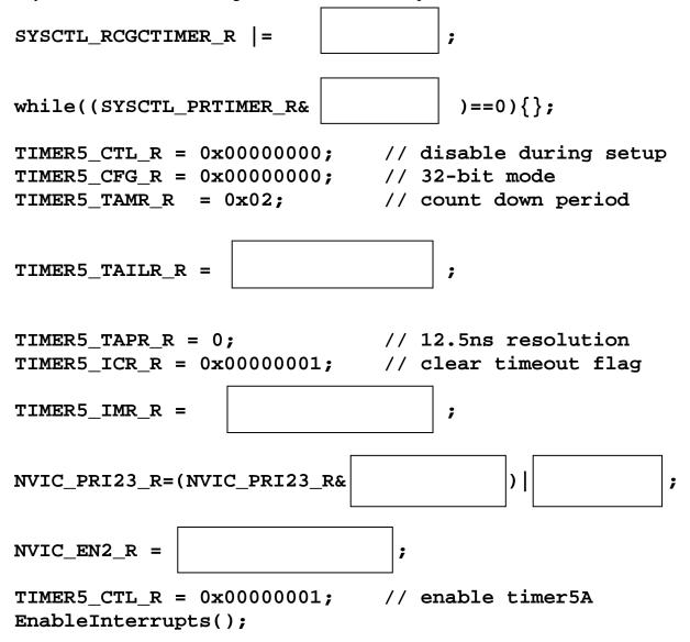
The **SYSCTL\_PRTIMER\_R** register has one bit for every bit in the **SYSCTL\_RCGCTIMER\_R**, which is one if the corresponding clock bit is on and stable, and zero if the corresponding clock is off or unstable.
