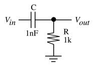
(5) Part b) Draw a rough plot of the gain  $(|V_{out}/V_{in}|)$  versus frequency for the circuit. Include three points,  $f=0, f_c$  (the point where is gain is sqrt(2)/2=0.707), and at very large f. What is the value of  $f_c$ ?
