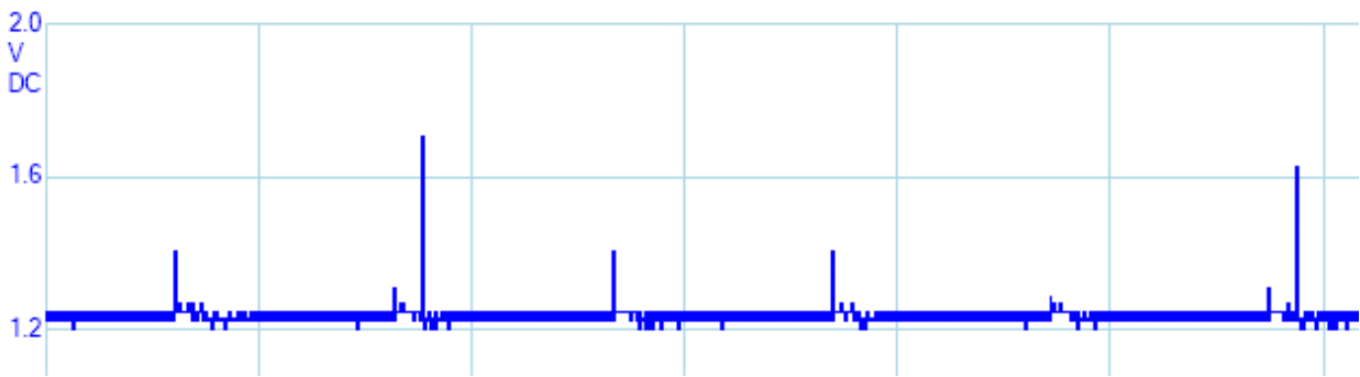
Figure 6.2. GPY0A21YK sensor output, distance=20 cm, DC mode, voltage scale is 0.4 V and time scale is 1 ms.
