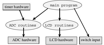
Figure 1.6. A call flow graph for a simple thermometer.
