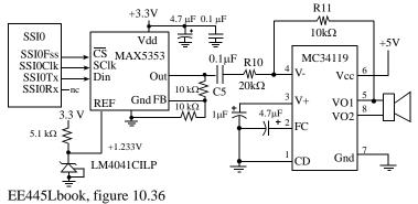
Need an audio amp to connect DAC output to  $32\Omega$  speaker Be careful to limit voltage and power to speaker  $\begin{array}{l} 0 < V < 5V \\ P < 200 \ mW \\ \textbf{0.2 W} > (V_{\rm O1}\text{-}V_{\rm O2})^2/32\Omega \\ \textbf{0.2 W} > (V_{\rm O1}\text{-}V_{\rm O2})^2/8\Omega \end{array}$
