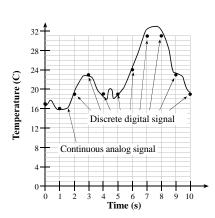
Nyquist theory states that if the signal is sampled at  $\mathbf{f}_{\mathbf{s}}$ , then the digital samples only contain frequency components from 0 to  $\frac{1}{2}\mathbf{f}_{\mathbf{s}}$ .
