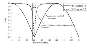
Figure 5.14. Gain versus frequency response of two 60 Hz digital notch filters.
