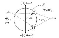
Figure 5.13. Pole-zero plot of a 60 Hz digital notch filter.
