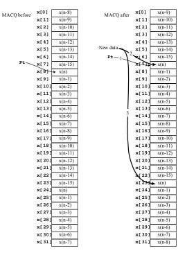
Figure 5.9. When data is put into a multiple access circular queue, the oldest data is lost.
