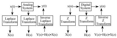
Figure 5.2. A transform can also be used to study a system in the frequency domain.
