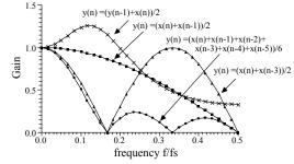
Figure 5.10. Gain versus frequency response for four simple digital filters.
