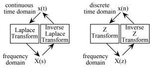
Fig 5.1 A transform is used to study a signal in the frequency domain.
