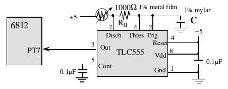
Part a) Assume the TCNT is running at 4MHz, therefore its period is 250ns. What is the largest period that can be measured with a single channel of input capture?
