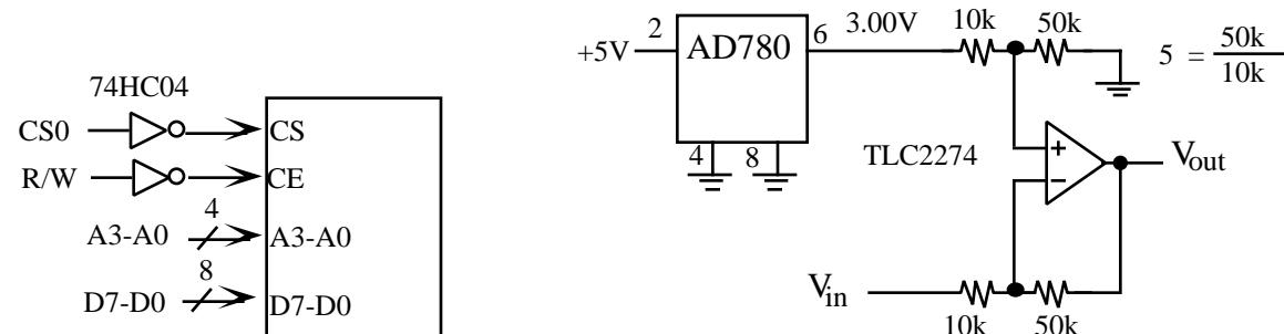
**(40) Question 3.** Interface an Output chipPart a)  $WDA = (106, t_{cyc} + 20)$ Part b)  $WDR = (\text{earlier}(CS-150, CE-150), \text{earlier}(CS, CE))$
