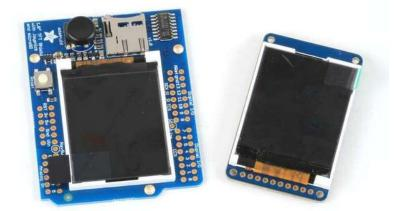
The 1.8" display has 128x160 color pixels. Unlike the low cost "Nokia 6110" and similar LCD displays, which are CSTN type and thus have poor color and slow refresh, this display is a true TFT! The TFT driver (ST7735R) can display full 18-bit color (262,144 shades!). And the LCD will
