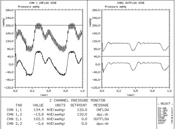
Figure 2. Real time graphics display for dual channel pressure monitor.
