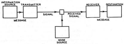
Fig. 1-Schematic diagram of a general communication system.
