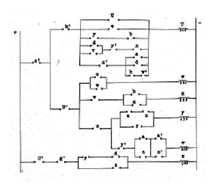
Electric Combination lock circuit
