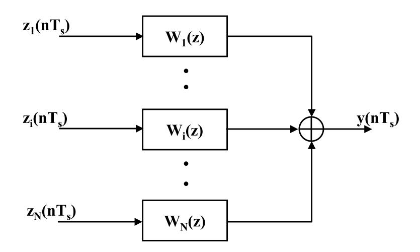
Fig. 1. Broadband Beamformer
