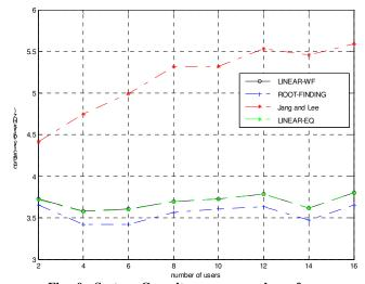
Fig. 0: System Capacity versus number of users. The capacity for Jang and Lee is much higher
