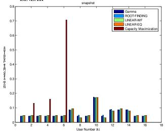
Fig. 3: A snapshot of rate proportion for a channel realization. Jang and Lee method distribute the capacity to user 2,4 and 6 only. LINEAR(WF, EQ) and ROOTFINDING share according to rate proportions
