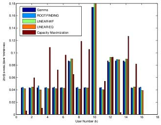
Fig. 2: Normalized Rate Proportion for 16 users. LINEAR(WF & EQ) and ROOTFINDING methods give fair share of the system capacity to the users. LINEAR
