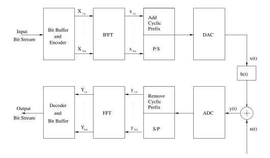
Figure 1: Block Diagram of the DMT transceiver (P/S and S/P mean parallel-to-serial and serial-to-parallel converters, respectively) [5]
