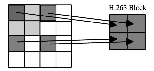
4x4 IDCT computed of upper left corner of each block. Four of these put together make up single block in H.263 macroblock.
