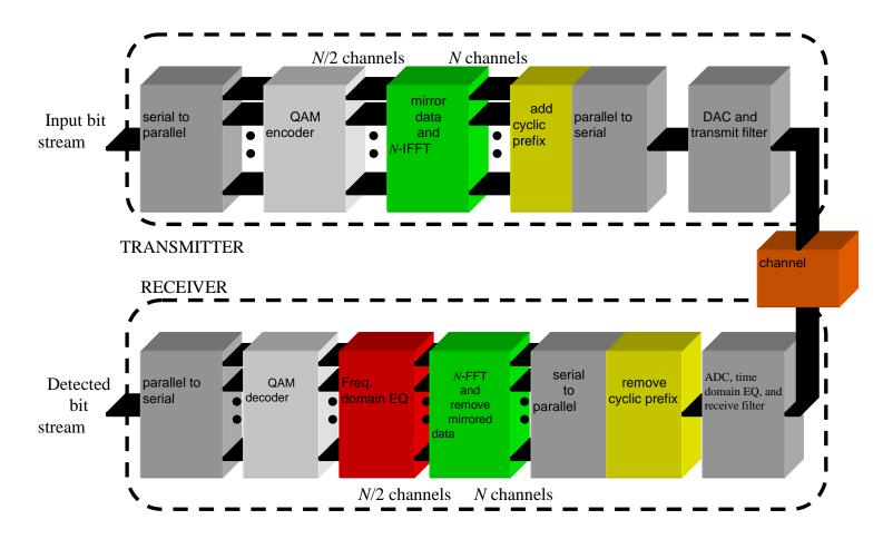
A block diagram of an ADSL transceiver
