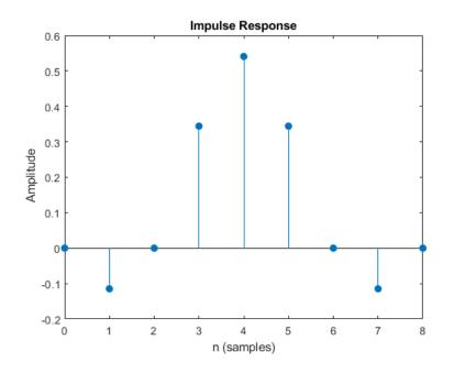
Before using freqz, we need to specify how many points 'n' to sample the DTFT in the interval [0,  $\pi$ ). For this example, we will choose n so that we have 1 Hz resolution.
