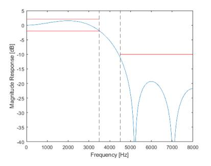
Visually, it appears to meet the specification, but it appears to be close to violating the passband ripple condition (at 3500 Hz, the red line is very close to touching the blue line.) We can use the vectors h and f returned from freqz to explicitly check the condition at every 1 Hz interval:
