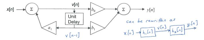
(a) Is this a finite impulse response filter or an infinite impulse response filter? Why? 4 points.
