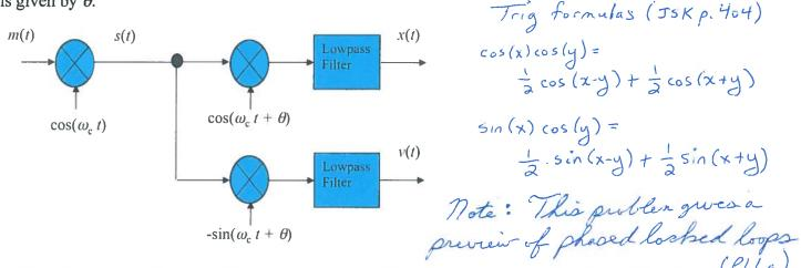
Assume the lowpass filters are ideal and have a gain of 2. Please ignore the delay through the filters.
