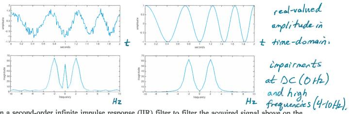
Design a second-order infinite impulse response (IIR) filter to filter the acquired signal above on the left to give the sinusoidal signal above on the right
