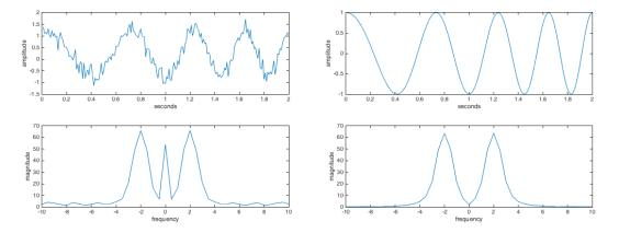
Design a second-order infinite impulse response (IIR) filter to filter the acquired signal above on the left to give the sinusoidal signal above on the right
