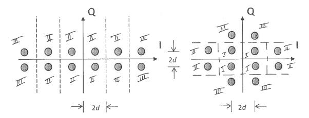
Energy in the pulse shape is 1. Symbol time  $T_{\text{sym}}$  is 1s. The constellation on the left includes the decision regions with boundaries shown by the I axis, Q axis and dashed lines.
