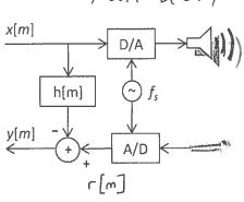
The analog-to-digital (A/D) and digital-to-analog (D/A) converters are synchronized by use of a common sampling clock. The A/D and D/A converters quantize to B bits per sample.
