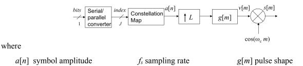
J bits/symbol L samples/symbol  $\omega_c$  carrier frequency
