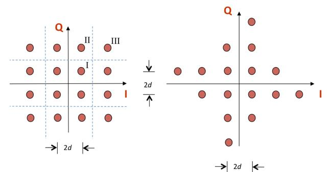
Energy in the pulse shape is 1. Symbol time  $T_{sym}$  is 1s. The constellation on the left includes the decision regions with boundaries shown by the in-phase (I) axis, quadrature (Q) axis and dashed lines.
