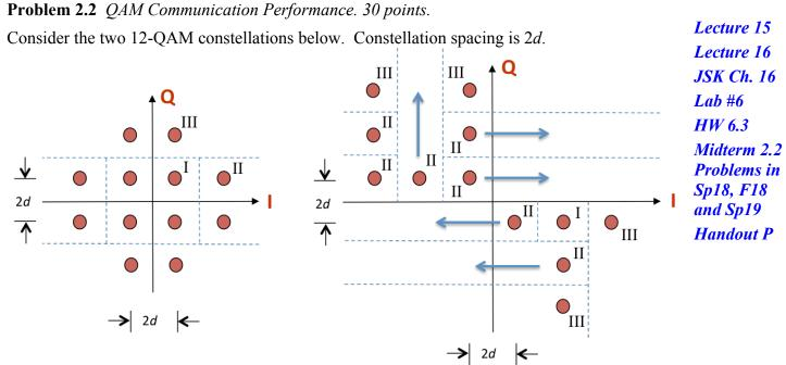
Energy in the pulse shape is 1. Symbol time  $T_{sym}$  is 1s. The constellation on the left includes the decision regions with boundaries shown by the in-phase (I) axis, quadrature (Q) axis and dashed lines.
