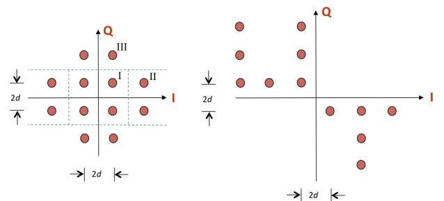
Energy in the pulse shape is 1. Symbol time  $T_{sym}$  is 1s. The constellation on the left includes the decision regions with boundaries shown by the in-phase (I) axis, quadrature (Q) axis and dashed lines.
