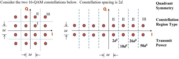
Energy in the pulse shape is 1. Symbol time  $T_{sym}$  is 1s. The constellation on the left includes the decision regions with boundaries shown by the in-phase (I) axis, quadrature (Q) axis and dashed lines.
