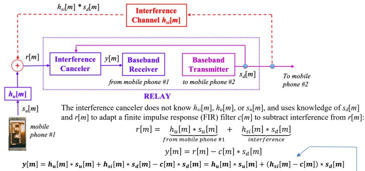
(a) What objective function would you use? Why? 8 points. Adapt canceler to remove interference in r[m] and hence reduce its power:  $J(y[m]) = \frac{1}{2} y^2[m]$ . Best removal when  $c[m] = h_{si}[m]$ .
